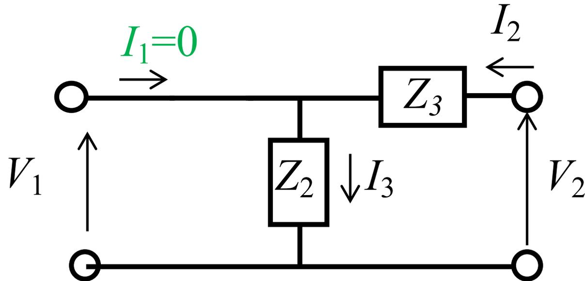
$$V_1 = \frac{Z_2}{Z_2 + Z_3} V_2 = Z_2 I_2 \quad \therefore \quad z_{12} = \frac{V_1}{I_2} = Z_2$$
