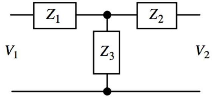
$$\begin{pmatrix} Z'_{11} & Z'_{12} \\ Z'_{21} & Z'_{22} \end{pmatrix} = \begin{pmatrix} Z_1 + Z_3 & Z_3 \\ Z_3 & Z_2 + Z_3 \end{pmatrix} \quad \left. \begin{array}{l} Z_1 = j\omega(L_1 - M) \\ Z_2 = j\omega(L_2 - M) \\ Z_3 = j\omega M \end{array} \right\}$$
