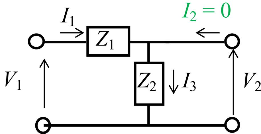
$$V_1 = (Z_1 + Z_2)I_1 \quad \therefore \quad z_{11} = \frac{V_1}{I_1} = Z_1 + Z_2$$
