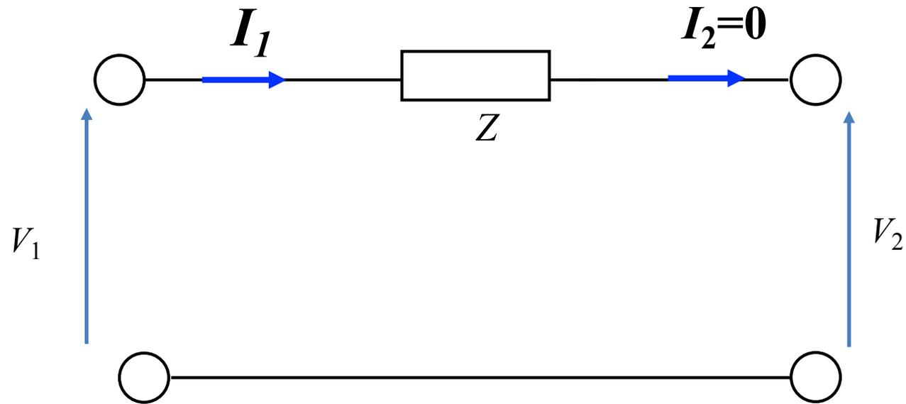
$$C = \left. \frac{I_1}{V_2} \right|_{I_2=0}$$
