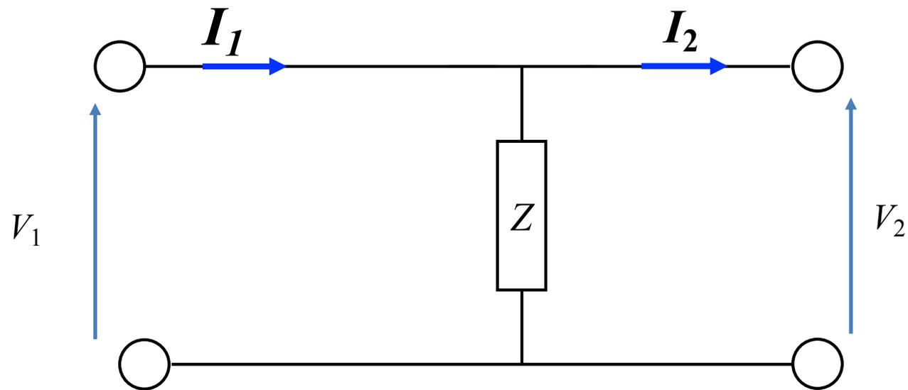
$$D = \left. \frac{I_1}{I_2} \right|_{V_2=0}$$
