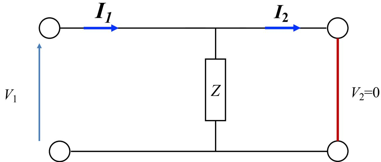
$$B = \frac{V_1}{I_2} \Big|_{V_2=0}$$
