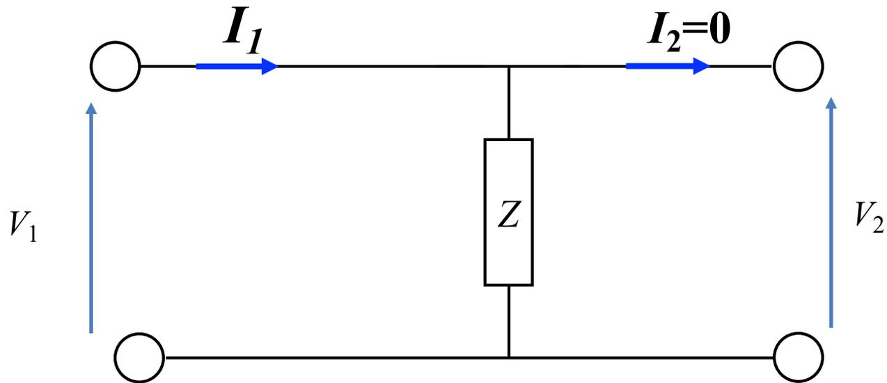
$$A = \left. \frac{V_1}{V_2} \right|_{I_2=0}$$
