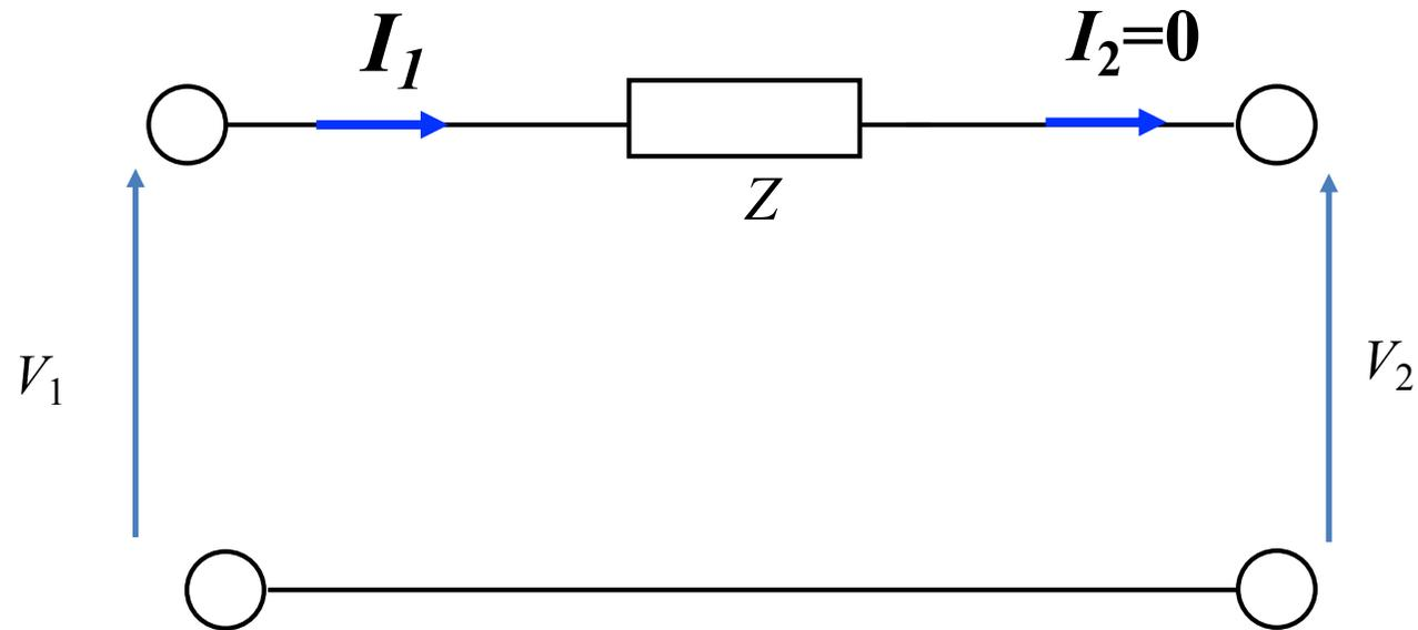
$$A = \left. \frac{V_1}{V_2} \right|_{I_2=0}$$
