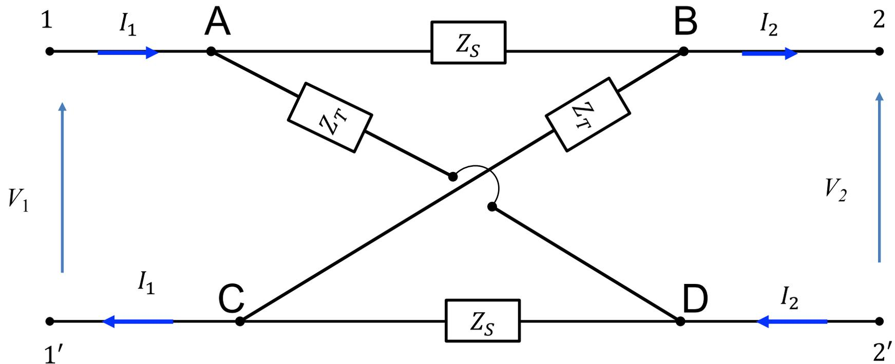
$$A = \left. \frac{\dot{V}_1}{\dot{V}_2} \right|_{I_2=0} = \text{出力端開放 電圧転送比}$$
