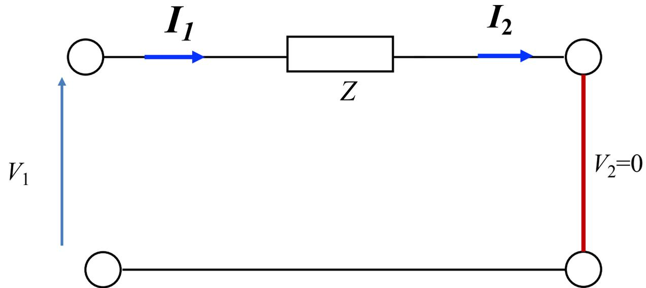
$$B = \left. \frac{V_1}{I_2} \right|_{V_2=0}$$
