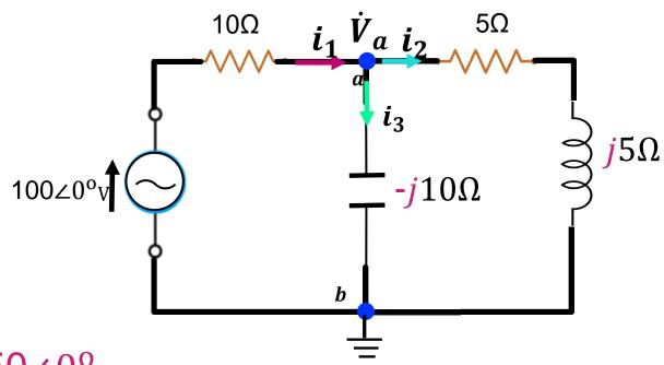
$$i_2 = \frac{50 \angle 0^{\circ}}{5 + j5} = 5 \angle 0^{\circ} (1 - j) = 5 \angle 0^{\circ} * 1.414 \angle -45^{\circ}$$
