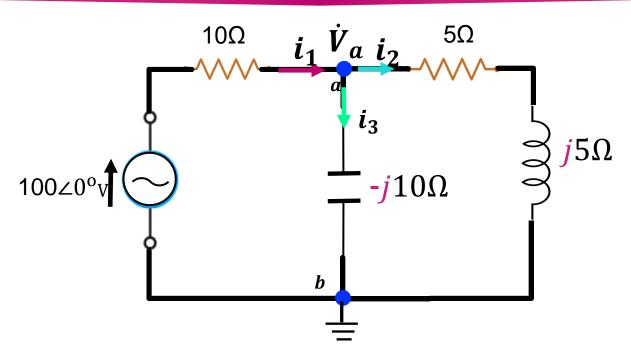
$$i_1 = \frac{100 \angle 0^{\circ} - 50 \angle 0^{\circ}}{10} = 5 \angle 0^{\circ} A$$
