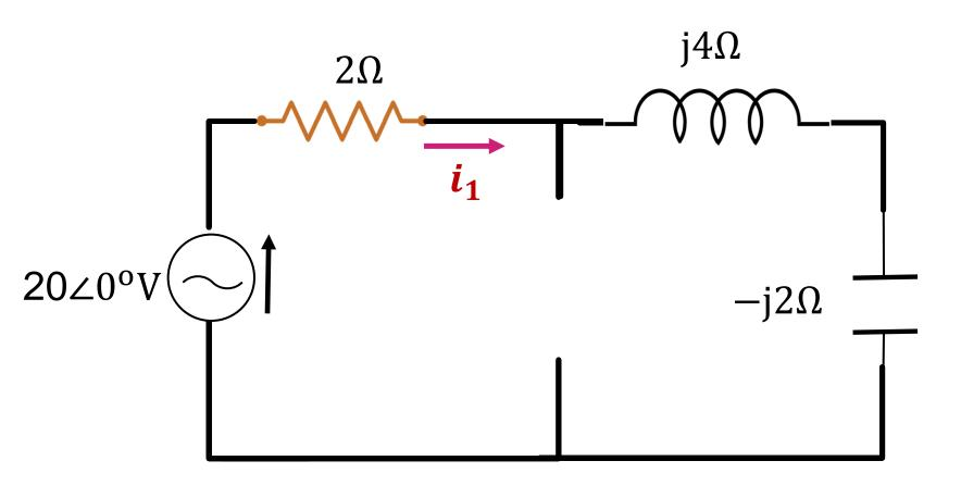
$$i_1 = \frac{20 \angle 0^{\circ}}{2 + j2} = 5(1 - j) = 7.07 \angle -45^{\circ}$$
