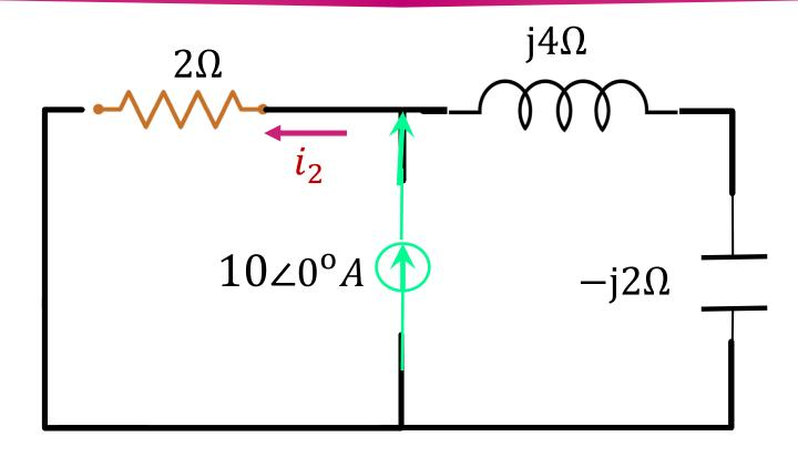
$$i_2 = \frac{2j}{2+j2} 8 \angle 0^{\circ} = \frac{1}{1-j} 8 \angle 0^{\circ} = 5(1+j) = 7.07 \angle 45^{\circ}$$
