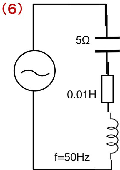
$$\dot{Z} = R + j\left(\omega L - \frac{1}{\omega C}\right) = \sqrt{R^2 + \left(\omega L - \frac{1}{\omega C}\right)^2} e^{j\varphi}$$
