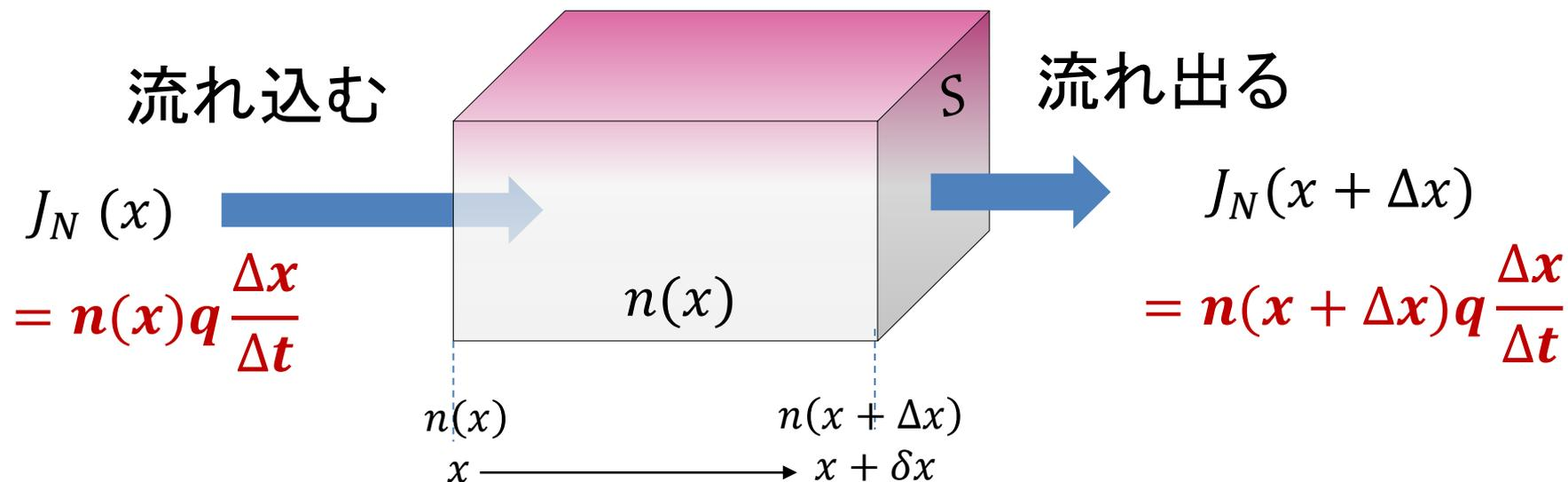
$$J_N(x) - J_N(x + \Delta x) = \{n(x) - n(x + \Delta x)\}q \frac{\Delta x}{\Delta t}$$
