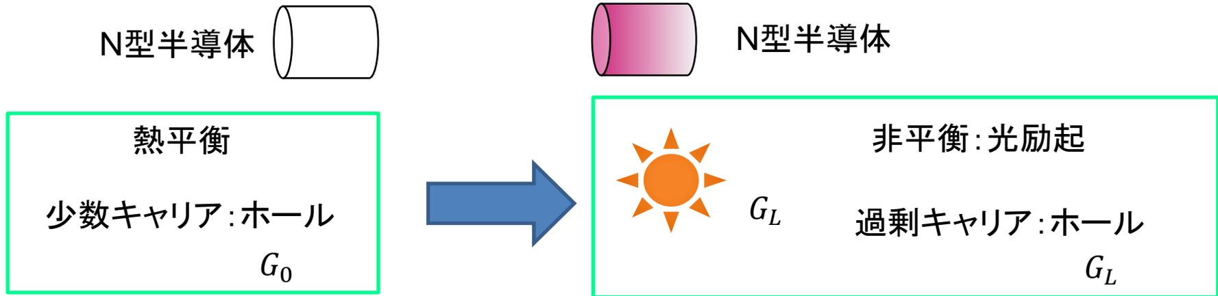
$$\frac{\partial p(x)}{\partial t} = G_L + G_0 - R + \frac{1}{-q} \frac{\partial J_N}{\partial x}$$
